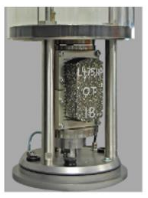
Texas Overlay Test
