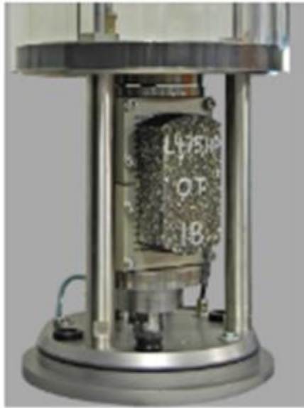
Texas Overlay Test
