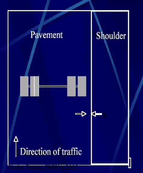
Used to calculate pavement responses & the number of axle load applications over a point for predicting distress & performance.
