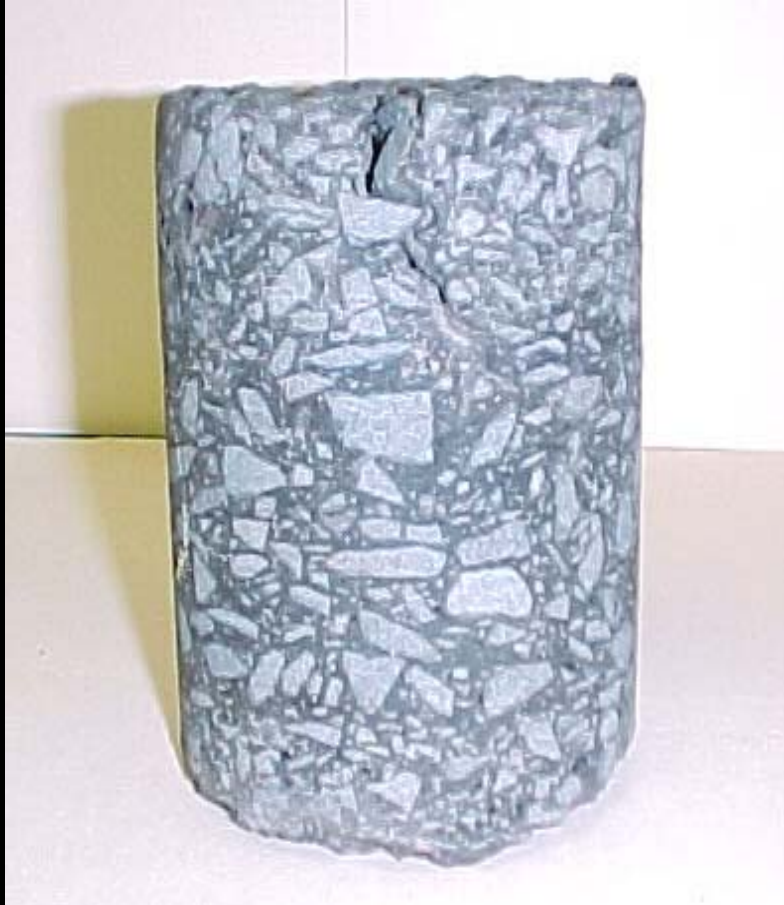
Top Down Cracking
