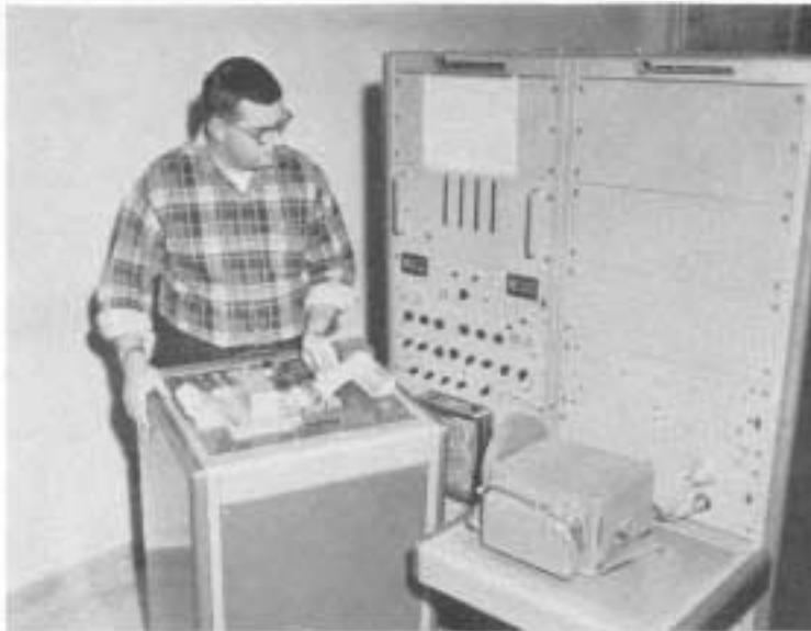
Figure 26. Chart reader used with longitudinal profilometer to transcribe information to punched paper tape.
